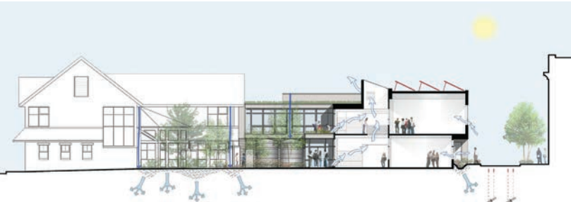
Daylighting is a key design strategy for the project with a skylit atrium enhancing classroom daylighting through borrowed light at the center of the building. Circulation spaces are naturally ventilated while mechanically cooled lab classrooms and offices have operable windows for swing seasons.
